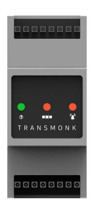
The device is made to sense the presence of water in any room/ environment. It is used to protect against flooding in server rooms, battery rooms, power rooms, offices, laboratories, special designed critical areas etc. It featured with a detector (fit inside panel) and a sensor (installed in critical area which needed to be avoided from any water). When the sensor meet water, it automatically activates the alarm on the detector, switching the status of the relay.
